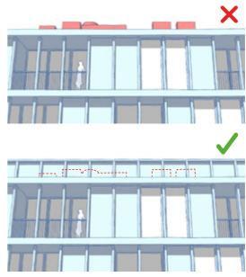
Fig.5.11 - Plant and services on roof. Seeing plant equipment from street level can have a negative impact on the character of the street.
